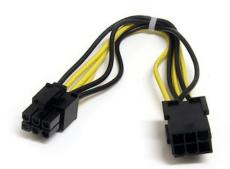
The PCIEPOWEXT 8-inch PCI Express Power Extension Cable extends the reach of your ATX12V power supply PCIe power connector by 8 inches, making it easier to power your PCI Express based video card without having to stretch or add strain to the PCI Express power connector from the power supply.
