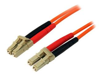
The 50FIBLCLC5 5m LSZH LC to LC Fiber Cable features 50/125 micron fiber for high-speed, high bandwidth data transmissions over Gigabit Ethernet and Fiber Channel networks, with support for duplex multimode applications.
