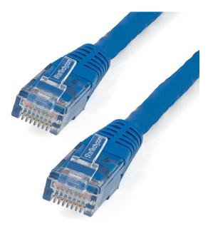
The C6PATCH50BL Cat 6 Patch Cable (50 ft) meets or exceeds all Category 6 cable specifications to ensure reliable Gigabit network connections, and features a durable blue PVC jacket that enables you to color code your network cable runs as needed.
