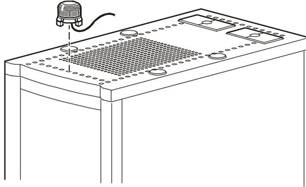
2. Route the beacon cable into the enclosure through one of the holes on the roof of the enclosure.
