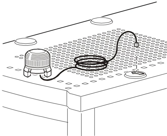
3. Plug the cable into the port marked **Alarm Beacon** on the rear panel of the Environmental Management System.
