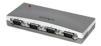
This 4 Port USB to RS232 Serial Hub lets you connect up to four RS232 serial devices to your Mac or PC laptop or desktop computer through a single USB port, as though the computer offered built-on DB9M serial connectors.
