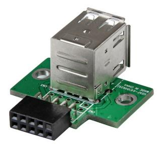
This USB A to USB Motherboard 4-Pin Header plugs directly into a motherboard USB header, providing two standard USB A female ports.
