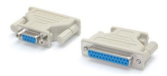
The AT925FF DB9F to DB25F cable adapter converts a 9-pin serial port into a 25-pin female port. Backed by StarTech.com's lifetime warranty.
