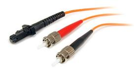
The FIBMTST1, 1-meter (3.3ft) Multimode 62.5/125 Duplex Fiber Patch Cable is terminated with one MTRJ (male) connector and one ST (male) connector, to provide the necessary connection between fiber networking devices for high-speed, long distance networks.
