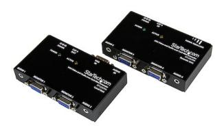
The ST122UTPA VGA Video Extender over Cat 5 with Audio allows up to 4 (2 local and 2 remote) monitors to be connected to a single PC. The video signal and corresponding audio are sent to the remote unit over standard 4 pair Category 5 or better (Cat 5e recommended) UTP cable, supporting extended video distances of up to 150m / 500ft.
