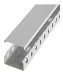
StarTech.com's AD105X1 is a screwmounted, two-piece plastic wiring duct available in various sizes. The parallel openings on its walls make for easy customization and the snap-lid provides easy access to cables while maintaining a tidy appearance. The AD105X1 screws into walls to provide a protective channel for cables, keeping them out of the way to eliminate clutter.
