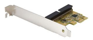
This PCI Express IDE Controller Adapter Card provides a cost-effective way to use legacy drives with modern computers, by converting a PCI Express port into an IDE port.
