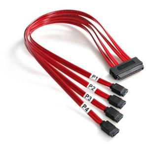
The SAS84S450 SFF-8484 to 4x SATA SAS cable features one 32-pin receptacle (SFF-8484) which fans out to four SATA 7-pin receptacles, providing a reliable solution for connecting up to four SATA HDDs to a SAS controller or backplane.
