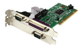
The PCI2S1P PCI Serial/Parallel Combo Card turns a PCI slot into two external 16C550 serial ports and one external EPP/ECP parallel port - an all-in-one solution that gives you both parallel and serial connections while taking up only one PCI slot.
