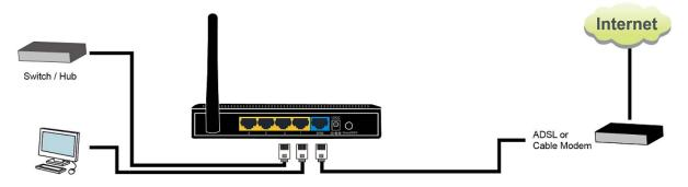
3. Insert the A/C power adapter into the wall socket, and then connect it to the 'Power' socket of the router.
