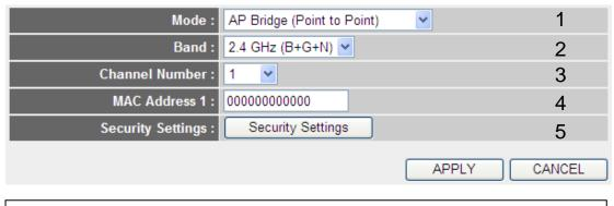
NOTE: The two wireless routers must use the same mode, band, channel number, and security setting!
