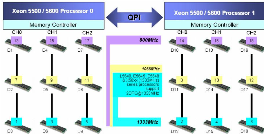
1-18: DIMM population sequence , D1-D18: DIMM slot assignments
