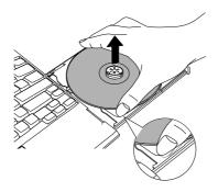
3. Push the center of the disc tray to close it. Press gently until it locks into place.
