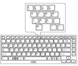
Figure 5-23The numeric keypad overlay
