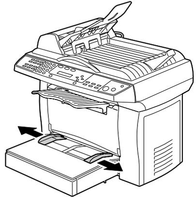
3 Insert the sheet of paper as far as possible into the manual feed tray with the side to be printed on facing up, and then adjust the paper guides so that both sides of paper are secure.
