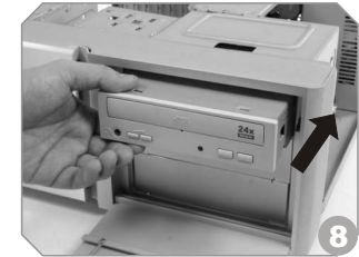
Remove the 5.25" drive bay cover. Then, insert the device into the 5.25" drive bay
