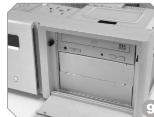
After placing 5.25" device, secure the device with screws
