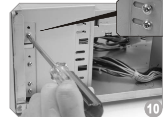
After placing 5.25" device, secure the device with screws
