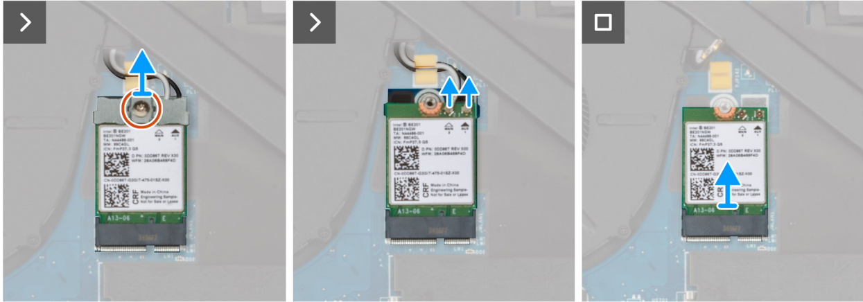
Figure 40. Removing the WLAN card
