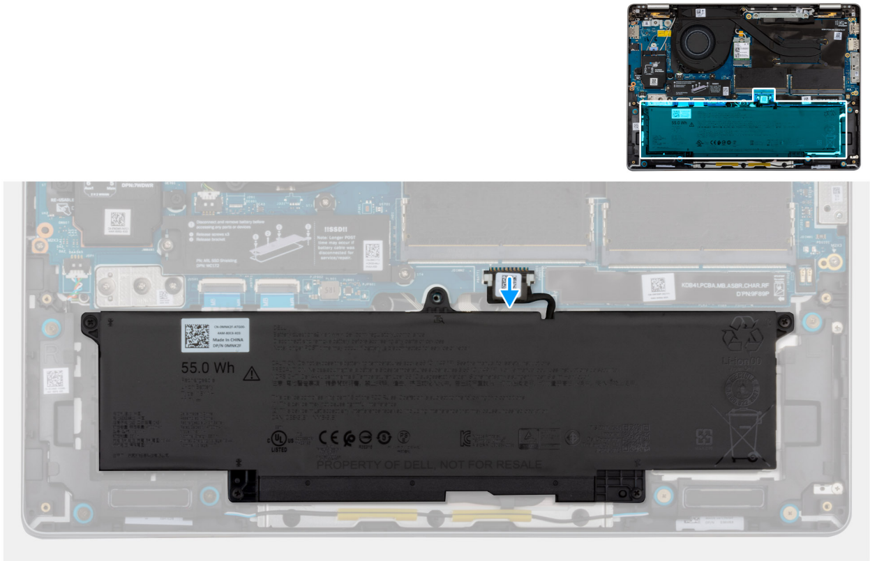
Figure 24. Disconnecting the battery cable
