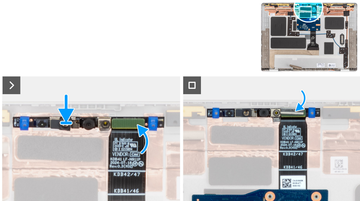
Figure 89. Installing the MIPI camera
