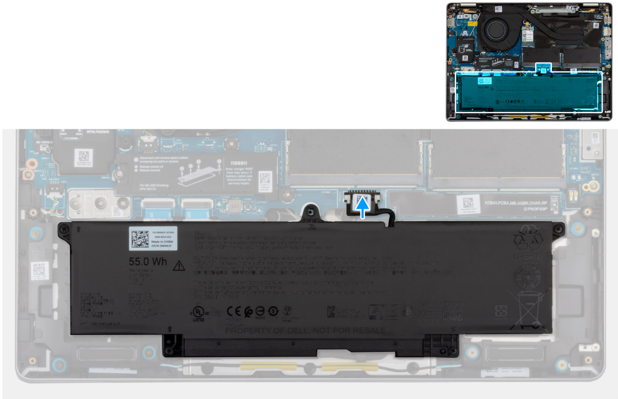
Figure 25. Connecting the battery cable
