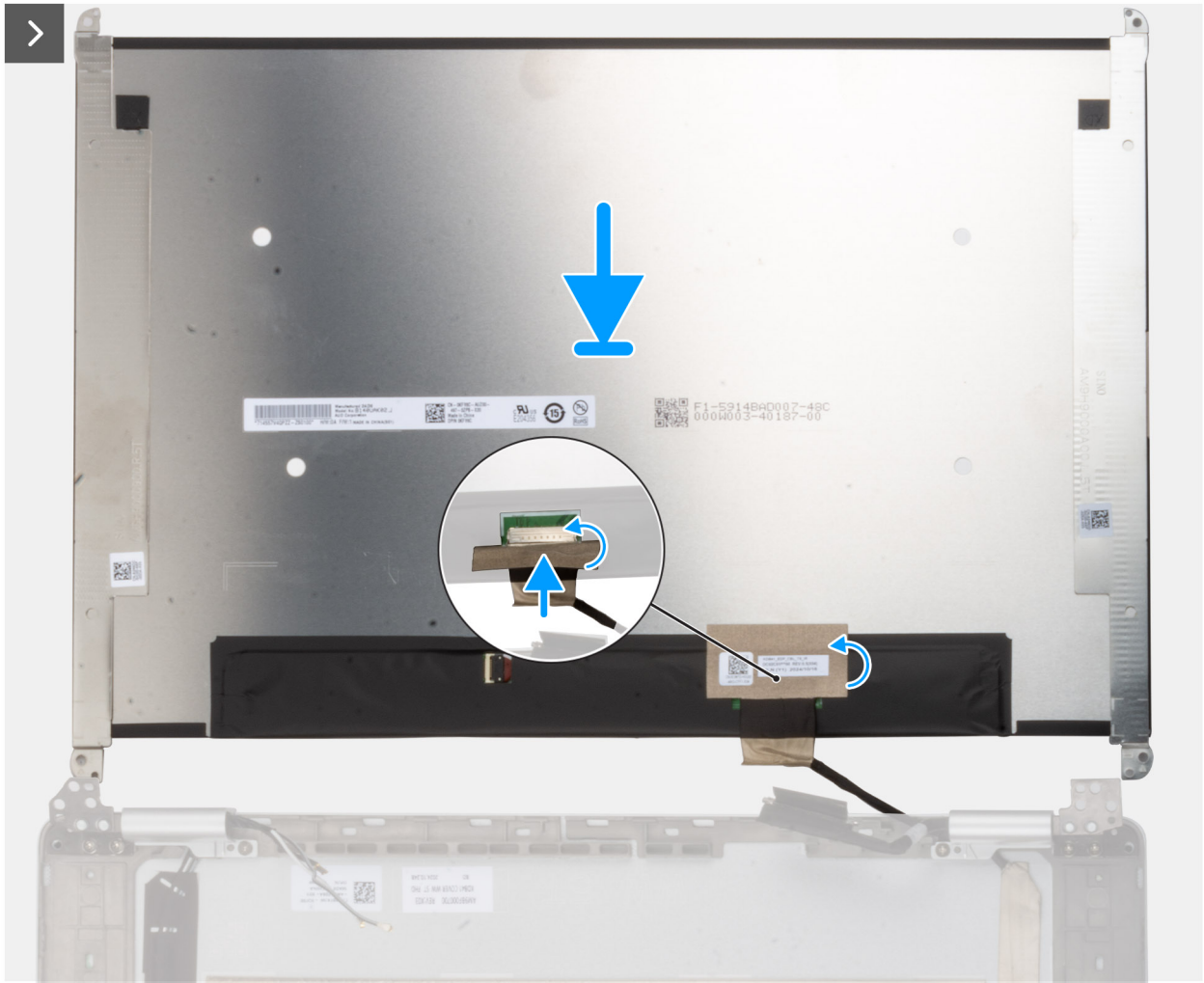
Figure 78. Installing the display panel
