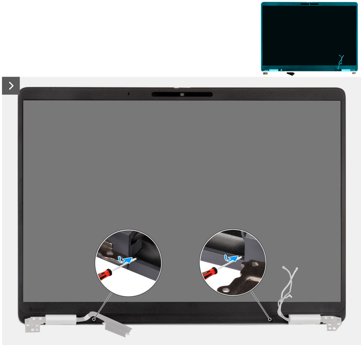
Figure 68. Removing the display bezel
