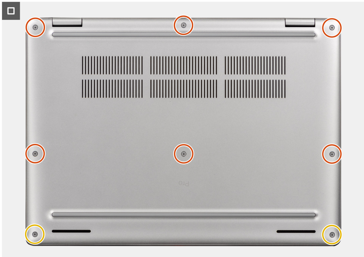
Figure 27. Installing the base cover
