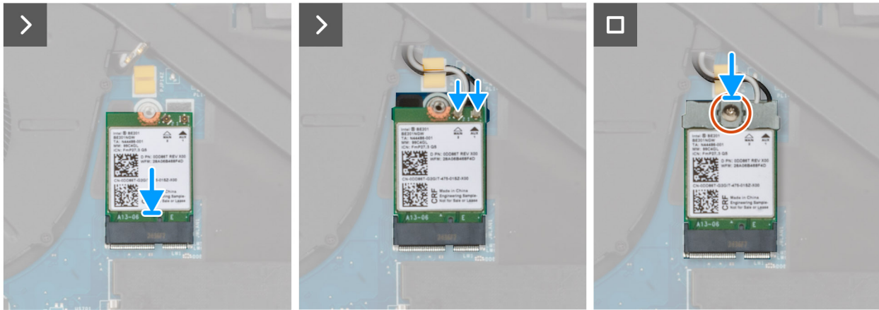
Figure 41. Installing the WLAN card
