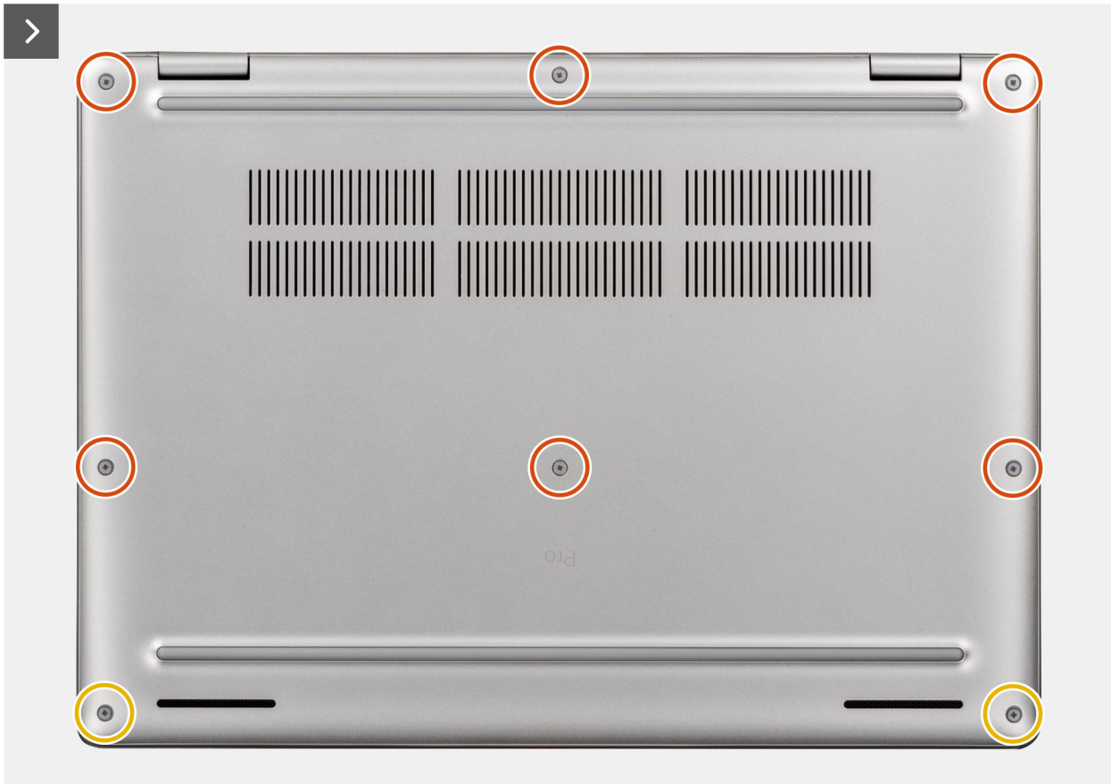
Figure 22. Removing the base cover
