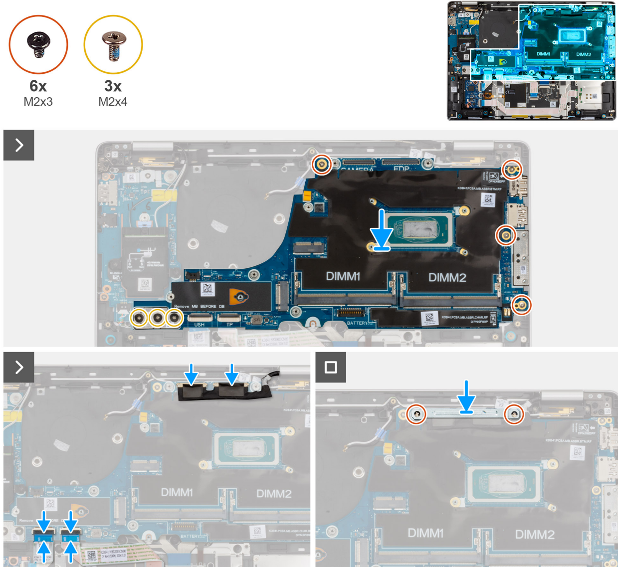
Figure 53. Installing the system board
