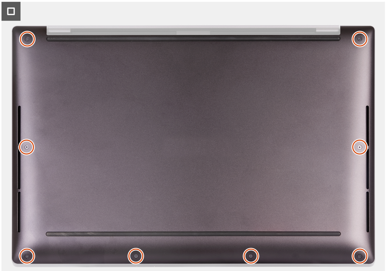
Figure 8. Tighten the eight screws that secure the base cover to the palm-rest assembly
