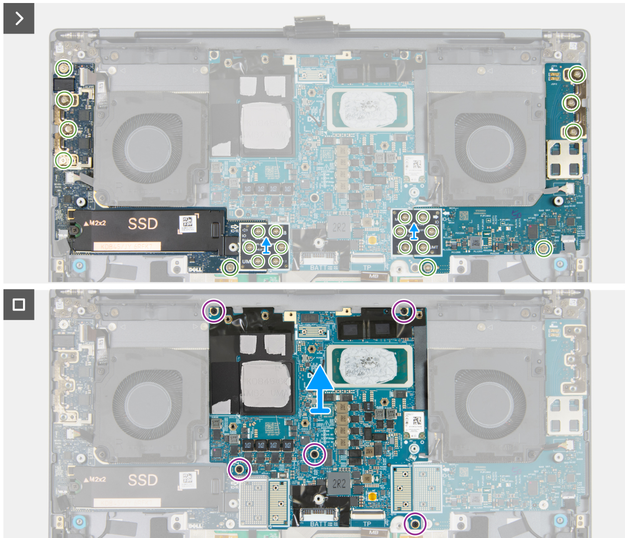
Figure 51. Removing the system board (integrated graphics)
