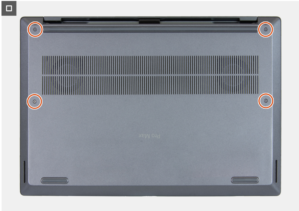
Figure 15. Installing the base cover
