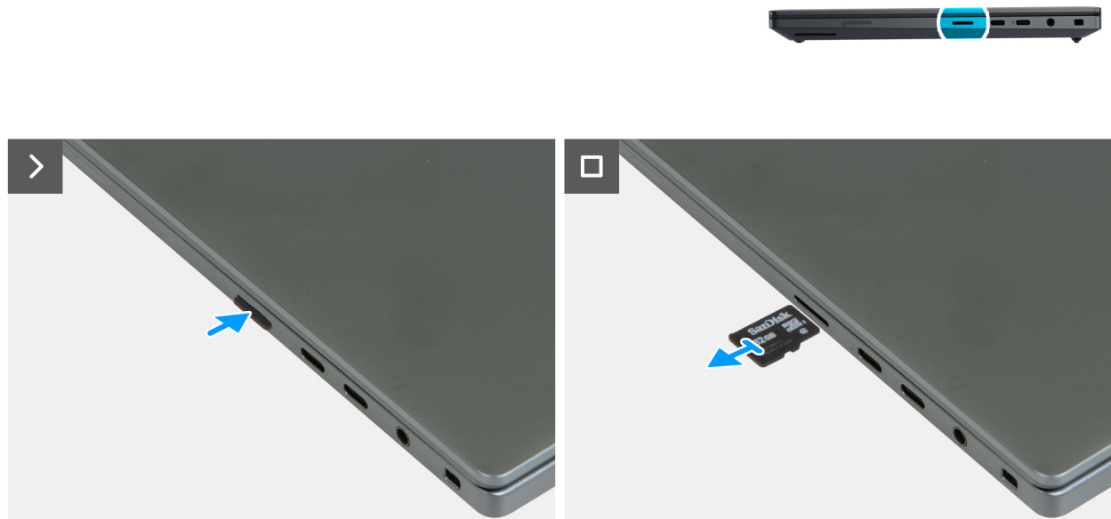
Figure 10. Removing the memory card
