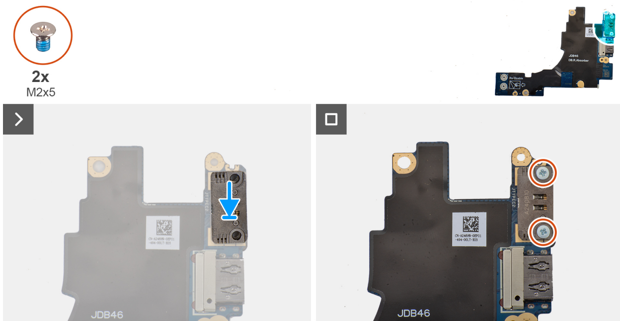
Figure 57. Installing the left USB Type-C module
