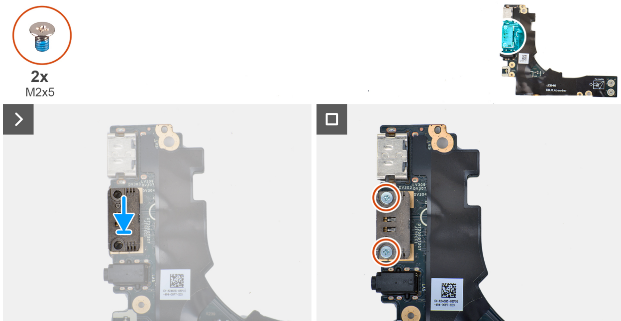
Figure 58. Removing the right USB Type-C module
