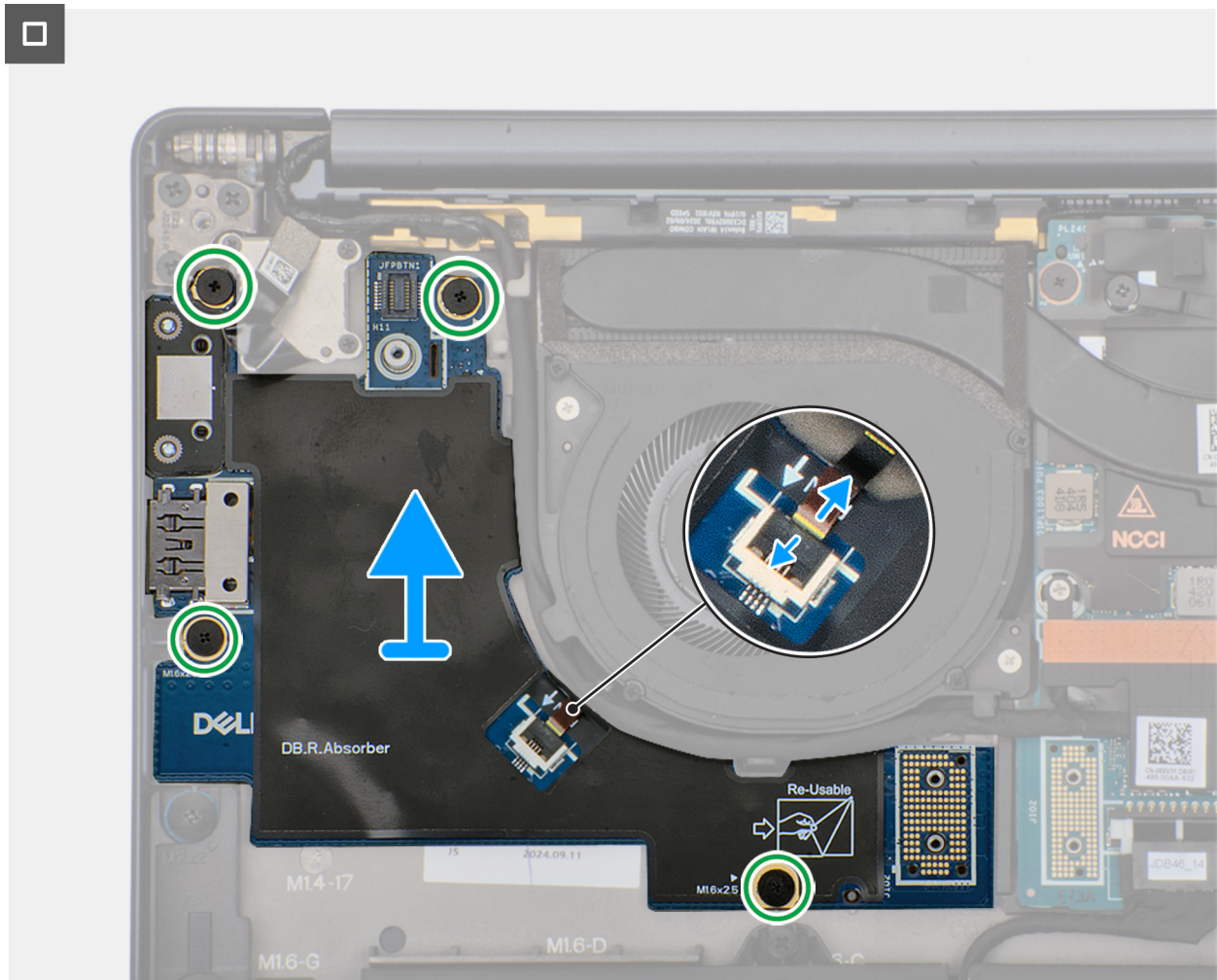
Figure 45. Removing the right I/O-board (without WWAN antennas)
