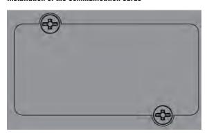
Accessory Slot: Remove the small cover panel from this slot to install optional accessories to remotely monitor and control your UPS. Refer to your accessory's manual for installation instructions. Contact <a href="mailto:tripplite.eaton.com">tripplite.eaton.com</a> for more information, including a list of available SNMP, network management and connectivity products.
