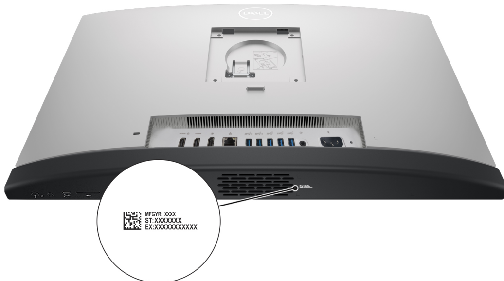
Figure 9. Service tag location of your OptiPlex All-in-One Plus 7420
