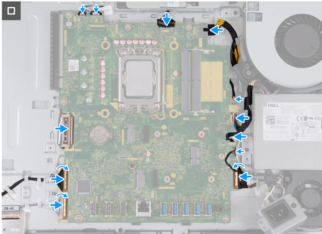
Figure 70. Installing the system board
