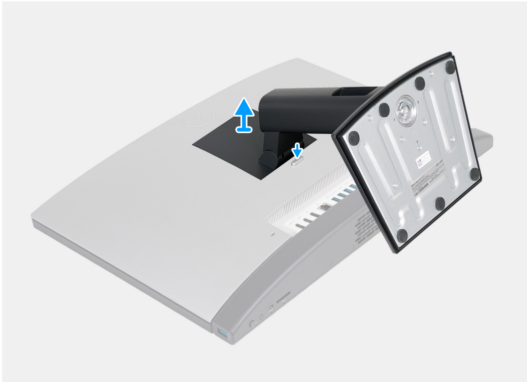
Figure 16. Removing the Fixed Stand
