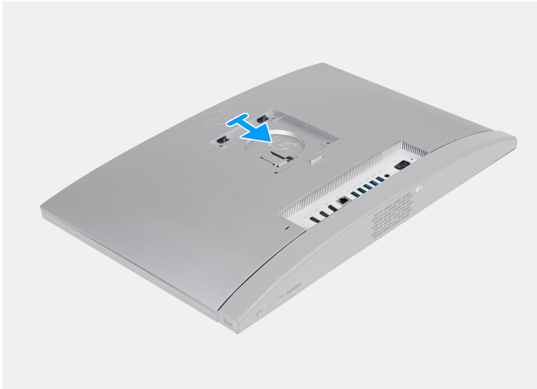
Figure 20. Installing the back cover
