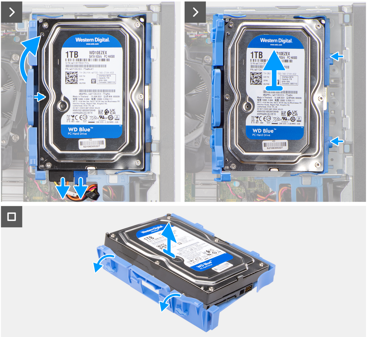
Figure 9. Removing the 3.5-inch hard drive
