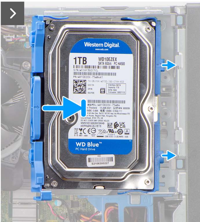
Figure 10. Installing the 3.5-inch hard drive
