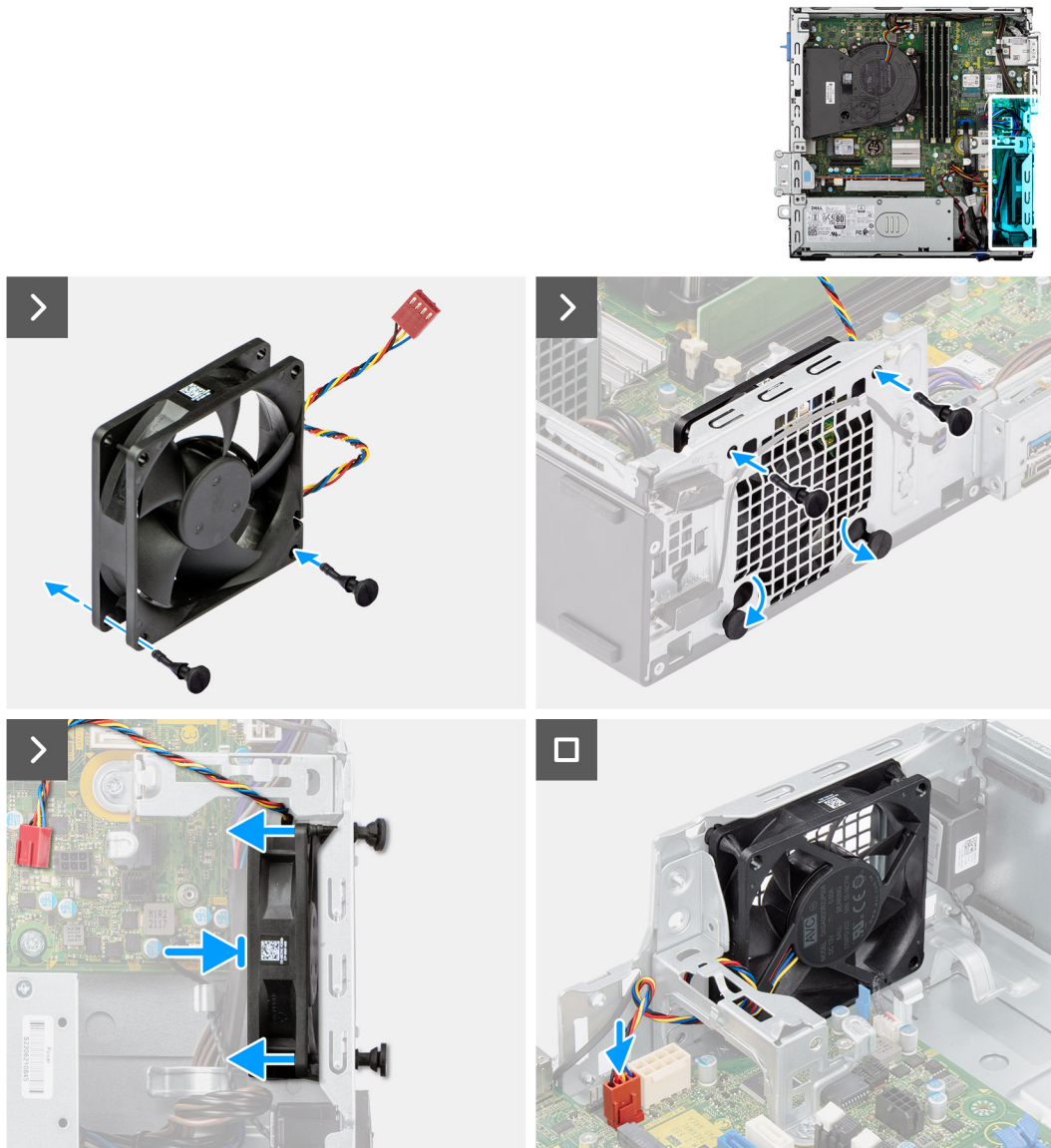
Figure 42. Installing the system fan
