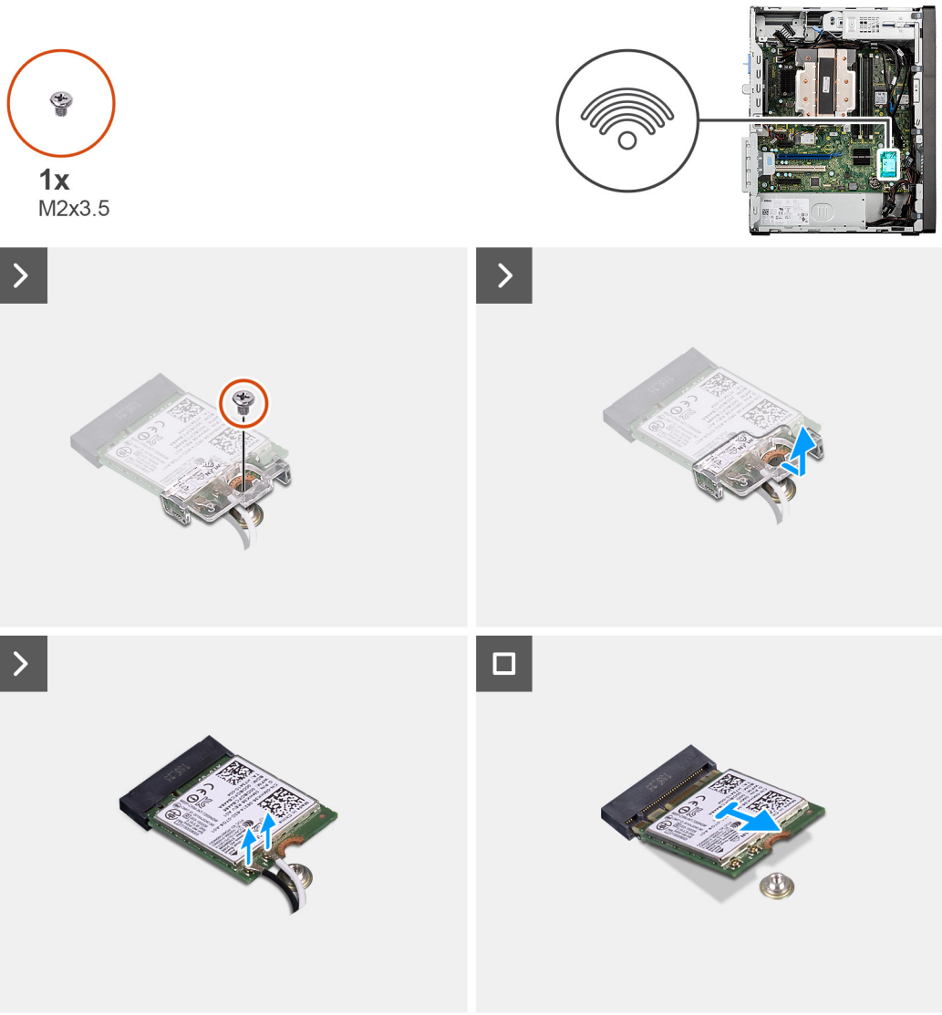
Figure 24. Removing the wireless card
