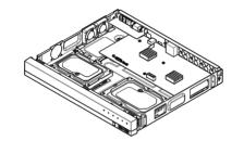
1 Loosen the screws on the back and slide the cover back to remove it.
