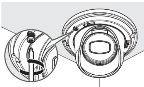
6. Put the middle cover back and rotate it clockwise until it is firmly in place.
