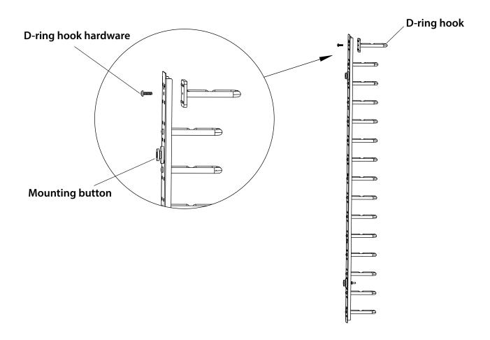
If your server rack lacks keyhole-shaped mounting holes, you will need to remove the mounting buttons or two D-ring hooks. Then, utilize the provided hardware to attach the cable organizer to your server rack.
