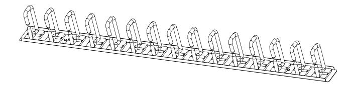
Vertical Cable Organizer with D-Ring Hooks - 6 ft ( 34" Length X2) Steel frame and Plastic Rings - Black
