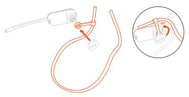
2 Choose the size and style of the eartip that fits most comfortably. Align the eartip with the notch facing the microphone as shown. Press on to attach.
