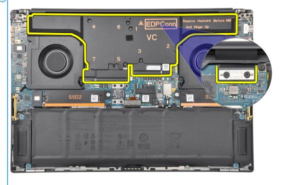
NOTE: Themal pads (thermal conductors) are on the heatsink. If the heatsink is replaced, the new heatsink is shipped with thermal pads. Ensure all thermal pads are in place between the heatsink and the system board.
