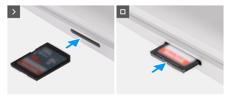
Insert the SD card into its slot until it click into place.
