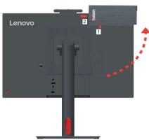
2. Screw the rear Wi-Fi antenna to the antenna connector on the rear of the computer. Then, adjust the angle of the antenna to 90 degrees.
