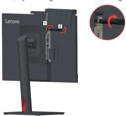
3. Pivot the cable cover as shown to the closed position.
