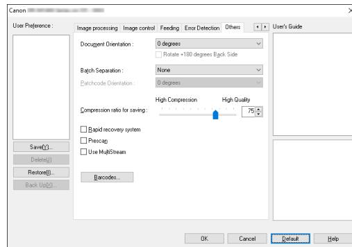
Configure special scan method and image processing settings.
