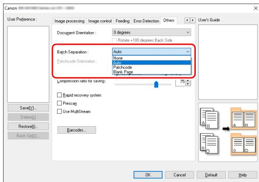
When [Batch Separation] is set to [Auto], the batch is separated after the next document is placed and scanning is continued.
