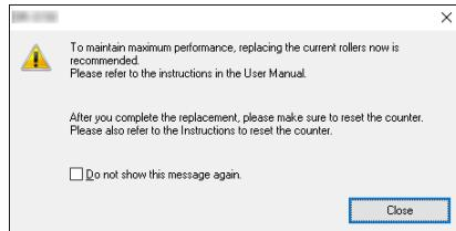
If this message begins to be displayed at startup, purchase an exchange roller kit and replace the worn parts with the consumable parts included in the kit (feed roller and retard roller). [See p. 64](#) for details about the exchange roller kit.
