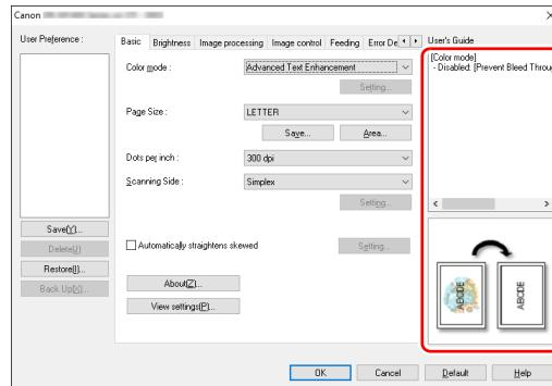
Informs you about the settings changed automatically by the driver. In addition, displays the image for which settings were currently made, in the illustrations.
