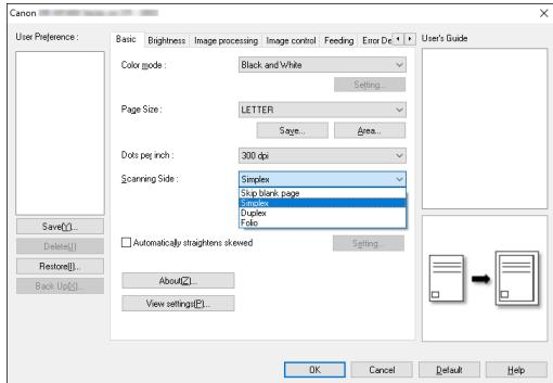
If the scanning side is set to [Skip blank page], the images of blank pages are deleted when images are saved.
