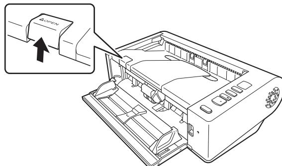
**3** Use compressed air to remove dust and paper particles from the inside of the scanner.
