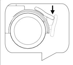
3A. Press the wheel lever up or down to place wheels in locked or unlocked mode depending if you want to be in a mobile or stationary setup. Make sure you adjust all (5) wheels at the same time or it won't properly be
