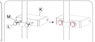
pole / floorstand (B) where you wish to attach the handle (K). Then align the screw and the U bracket (L,M) with the opening in the handle (K).
