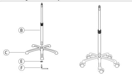
2A. Align the bottom of pole body (B) to the top center of the base (C). While pieces are connected, securely flip over so you can see the bottom. Align washer (E) to the hole on the bottom. Using your hands, identify L-shaped component (F) and rotate through the washer into the hole until securely tightened. Pole body and base should now be securely attached to each other.
