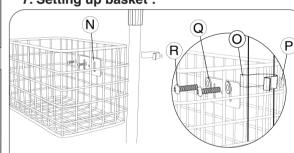
7A. Find the desired height on the pole / floorstand (B) Align U bracket (O) holes with basket (N) screw holes on either side of the central pole. Pass screw (R) through washer (Q), then through screw hole, and turn in nut (P) on opposite side
