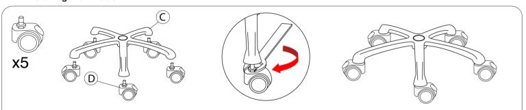
1A. Take one wheel (E) and align it to the leg arm holes on the underneath of the base (H). Initially you can use your hands and manually rotate the wheel until slightly tightened Then use the provided wrench tool (B) at the hex nut and rotate to securely tighten the rest of the way.
