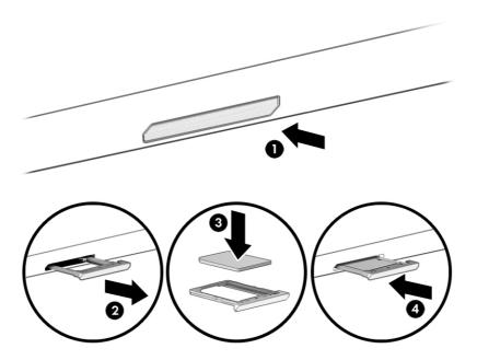
To remove the SIM card, press in gently on the SIM card access tray to disengage the SIM lock, and the tray pops out of the slot. Remove the SIM card. Replace the tray in the computer and press in gently on the tray until it is firmly seated.
