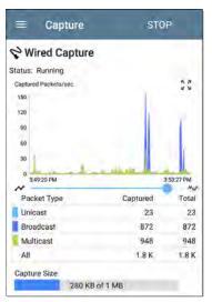
The Wired graph plots the type and number of packets being captured during the time the capture is running. By default, wired captures include Unicast, Broadcast, and Multicast packet types.
