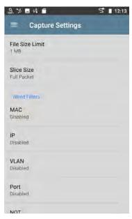
File Size Limit: Touch this field to specify a size for the capture file. The default size is 1 MB, and largest size allowed is 1000 MB. The capture
