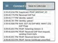
Select the action overflow icon at the top right on the Connect Log screen to attach the log to its associated AutoTest result on the Link-Live website. You can also attach the Connect Log from the floating action menu on the main Wired Profile screen.
