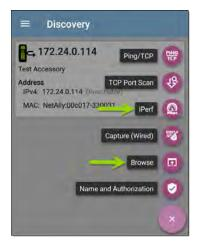
NOTE: You can select **Browse** in the floating action menu to open the Test Accessory's Web Interface, where you can view its status and configure its settings.
