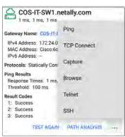
Touch blue links or the blue action overflow icon ••• at the bottom of the test results screens to run the Gateway TEST AGAIN, open another app, Browse to the Gateway's IPv4 Address, or start a Telnet or SSH session to the Gateway.
