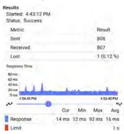
These graphs update in real time and save and display data for up to 24 hours (depending on test type and/or link status).
