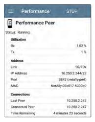
The screen displays real-time status, utilization, and rates for as long as the test is running.
