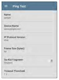
Name: This field allows you to assign a custom name to the test. The name appears on the target test card in the profile.
