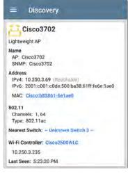
The Nearest Switch and Wi-Fi Controller links open a Discovery app Details screen for those devices
