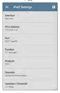
Touch each field to enter or revise selections as needed. Changed settings are automatically applied. When you finish configuring, tap the back button to return to the iPerf test screen.
