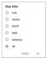
This setting directs the Wired Profile to stop testing after the selected test step. The excluded test cards will not appear on the Profile results screen.
