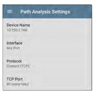
On the Path Analysis Settings screen, touch each field as needed to configure your target:
