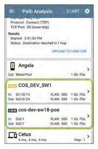
The LinkRunner is able to identify these Layer 2 switches and their interfaces because it has configured SNMP access to the switches.
