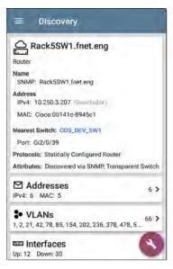
When a user opens the FAB and selects a different app, such as Path Analysis, only the address and name listed at the top of the Details screen will be populated in the Path Analysis app.
