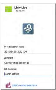
The Link-Live sharing screen for a screenshot or other image allows you to attach it to the most recently run (AutoTest, iPerf, or Cable) test result on the Results page, or just to the Uploaded Files page on Link-Live.com.
