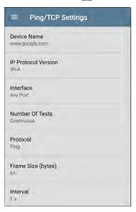
**Device Name**: Enter the IP address or DNS name of the target.
