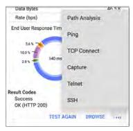
Touch blue links or the blue action overflow icon ••• at the bottom of the test results screens to run the HTTP TEST AGAIN, open another testing app, or Browse to the target address in your web browser.
