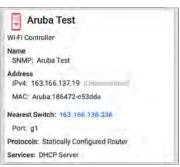
The top of the card shows the device type and icon (a Wi-Fi Controller with a **Failure or Error** status in the example image above).
