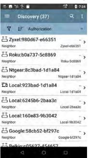
NOTE: Batch Authorization operates on the default MAC address of a device. If a device has multiple MACs, authorization will only be set on the default MAC address. Devices that do not have a discovered MAC address, such as unknown switches and off-net devices, cannot have an authorization setting.
