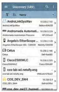
Like in AutoTest and other LinkRunner screens, the icons in Discovery change color to indicate a Warning or Failure condition. Discovery also displays device icons in Blue to indicate Problem-related information that does not constitute a warning or failure, and Green to indicate that a previous Problem has been resolved. (See the Problem Settings to adjust enabled Problems and thresholds.)
