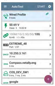
Like the main AutoTest screen, Wired Profile tests are summarized on cards. Touch a card to view individual test screens.
