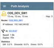
Tapping the <u>blue linked</u> switch name will open a <u>Discovery Details screen</u> for the switch, where the user can investigate the cause of the Warning.
