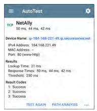
Device Name: DNS name of the device tested
