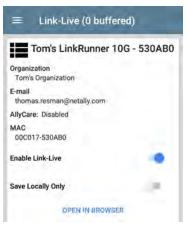
The "(# buffered)" in the Link-Live screen header indicates the number of files stored in the device memory when no active network connection is available. The buffered file types are listed below the main app card.
