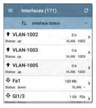
Like other Discovery list screens, the Interfaces list provides a number of Sort options, and the selected sort option affects the type of information displayed. The image above shows Interfaces sorted by Status (up or down). The image below shows Interfaces sorted by MAC Address, so each Interface's MAC address is displayed.
