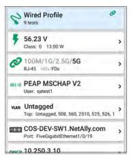
The 802.1X card only appears if the **802.1X** setting is enabled for the Wired Profile.
