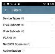
The Filters screen displays the number of devices or domains discovered for each category. Touch a category name to select filters by checking the boxes. The main Discovery screen will show only those devices or IDs that fall under your chosen filter parameters.
