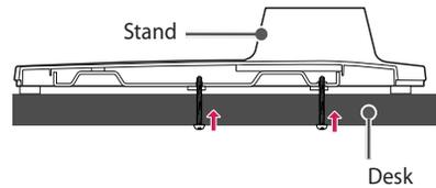
Screw: M5 x L (\*L: Table depth + 8~10 mm)
