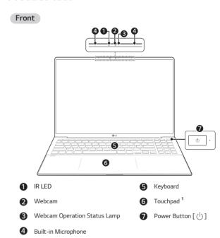
1 When using the touchpad while the product is turned on, LEDs are turned on on both sides. The external part of the touchpad LED cannot be used as a touchpad.
