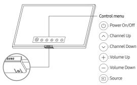
TV Controller button / Remote control sensor
