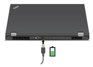
When the battery power is low, charge your battery by connecting your computer to ac power. Your ac power adapter supports the rapid charge function, the battery is 80% charged in about one hour when the computer is turned off. The actual charging time depends on the battery size, the physical environment, and whether you are using the computer.
