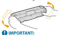
• Do not touch the surface of the drum on the bottom of the toner cartridge.
