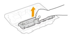
5 Shake the toner cartridge 5 or 6 times as shown below to evenly distribute the toner inside the cartridge.
