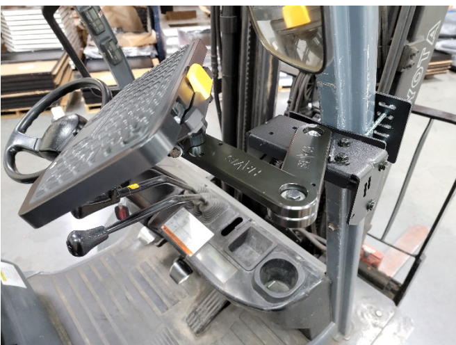
Add keyboard mount and keyboard to the MD-ARM-XXXX and confirm smooth movement.
