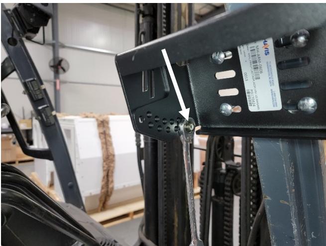
Remove the 1/4" x 3/4" bolt and nylock nut from both sides of the mount. Move mount until level.
