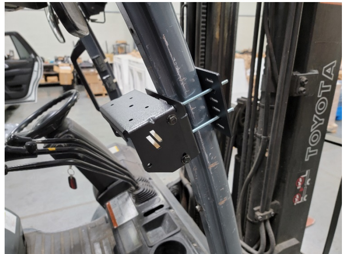
Place MH-ARM assembly on forward frame of forklift and determine desired height.
