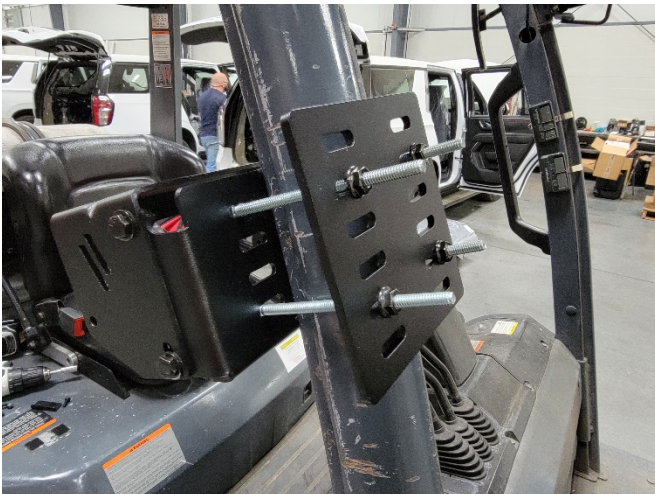
Place carriage bolts through assembly, back plate, and tighten nuts.
