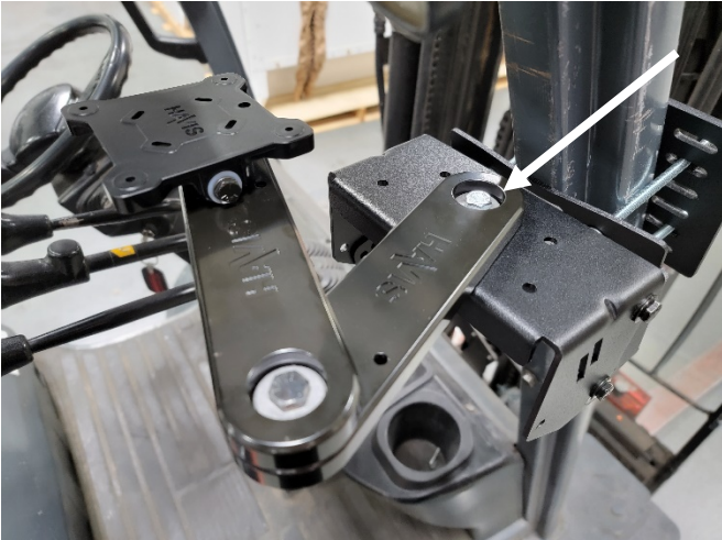
Mount the MD-ARM-XXXX to the top of the MH-ARM mount using supplied hardware.
