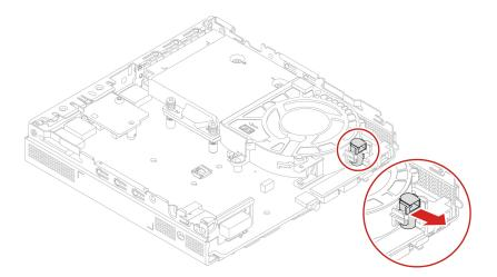
3. Disconnect the system fan cable from the system fan connector on the system board.
