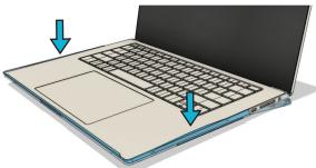
Slide the top case down **evenly (leveled)**, to secure the screen behind the side clips, until the device reaches the case's top edge.
