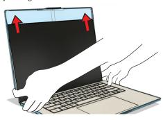
Gently push the rear clips down to unhook from the device.
