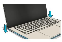
Push the left and right side clips down past the device, one side at a time, to release it from the bottom case.
