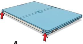
Start sliding the top case off by pushing up with your fingers on the bottom corners.
