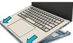
Align the device screen under the top case's side clips on both sides.
