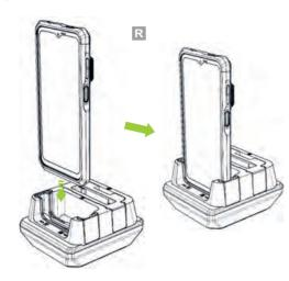
Insert an SKX6Pro without Protective Boot into the front and rear SKX6P-INSERT spacers. (V)
