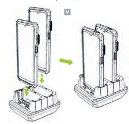
Insert the device with the metal buckle of the hand strap facing down as shown in the image below. (2)
