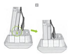
Insert SKX6Pro with Protective Boot into the SKX6P-BOOT spacer. (O)
