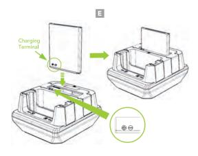
Insert XCover6 Pro with Samsung Case into the front spacer and XCover6 Pro with Samsung Case into the rear spacer. (I)
