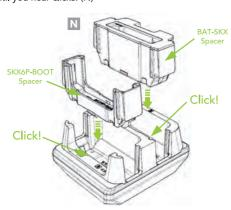
Insert SKX6Pro without Protective Boot into SKX6P-INSERT spacer, (R)
