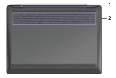
1. Ventilation slots (outlet) 2. Ventilation slots (inlet)
