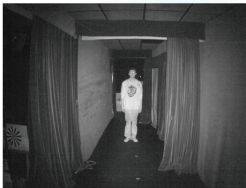
Smart IR enabled; distance: 3M
