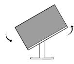
4 Complete the installation by rotating the monitor 90° clockwise and -90° counter clockwise as shown below.
