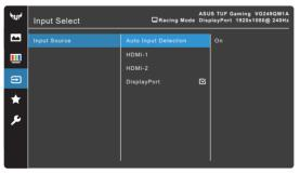
• **Auto Input Detection**: When enabled, the system will automatically select the latest inserted I/O port.
