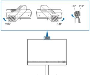
• Slide the webcam cover shutter on the top to open or close the lens.
